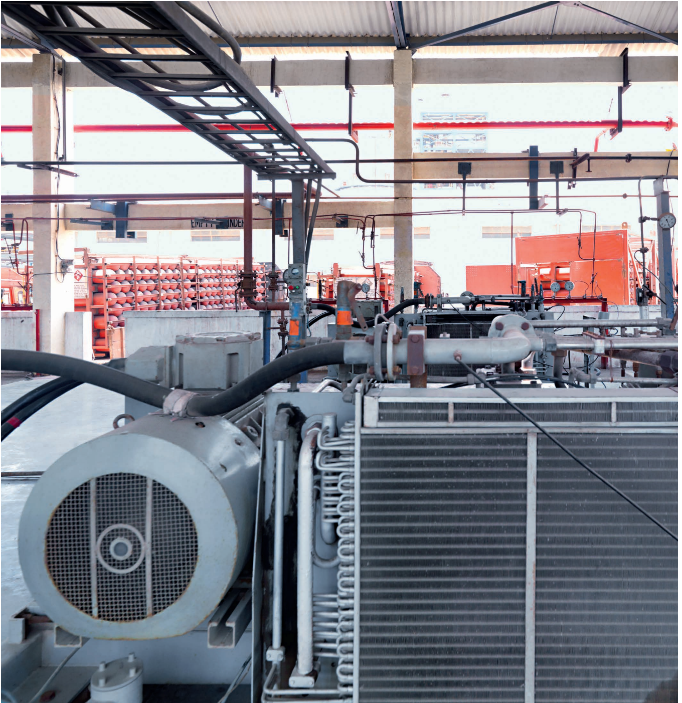
CU compressor meeting high safety standards in a hydrogen bottling plant
